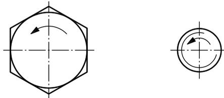
**Figure 17 — Examples of marking for left-hand thread**
