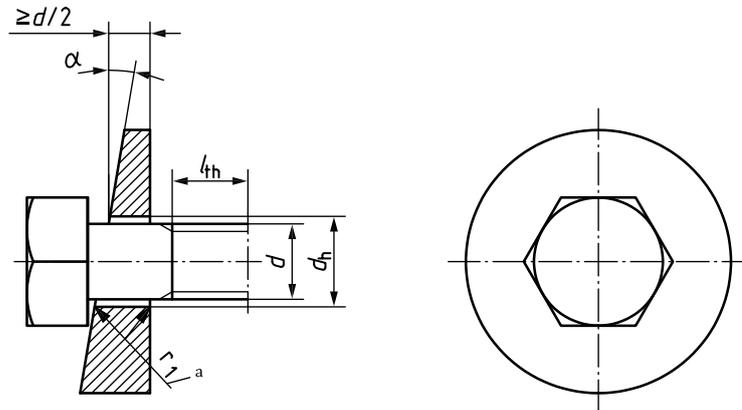
a Radius or chamfer of 45° (see Table 12).
