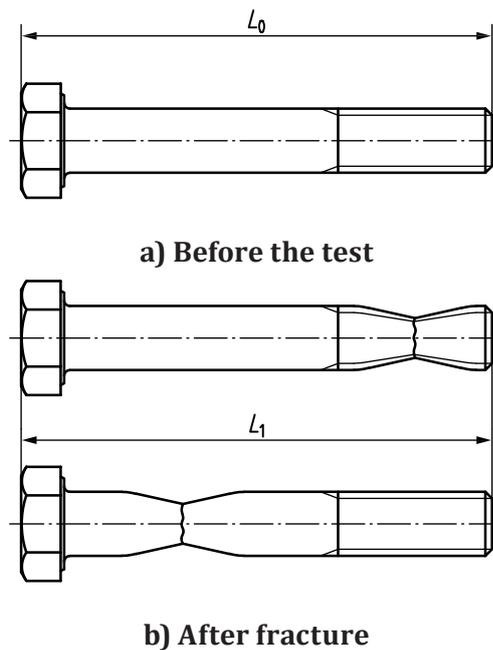
**Figure 6 — Determination of elongation after fracture,  $A$**
